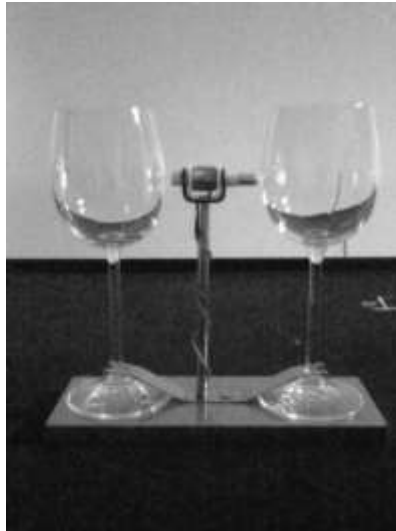
Figure 4: In this original doorbell, when electrical current flows through it, the coil becomes an electromagnet which forces the metallic core inside it to move, striking the glasses and producing a sound like two clinking glasses (Van der Jagt, 1994)
