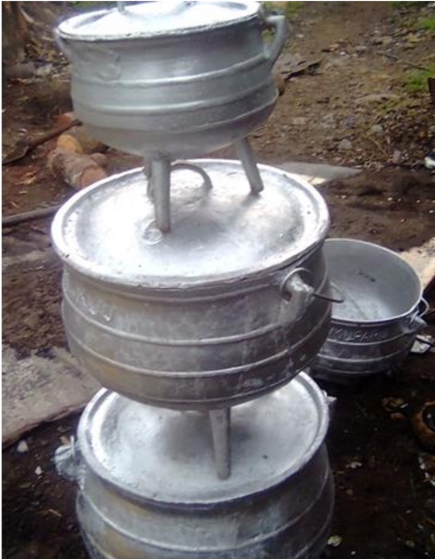
Figure 9: Cooking Pots from Recycled Aluminum Waste
