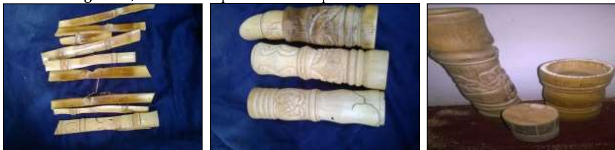
Figure 10, 11 & 12: Samples of bamboo preserved with neem leaf extracts
