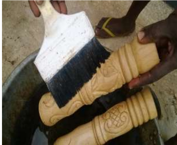
Figure 7: Painting the bamboos with neem leave extract
