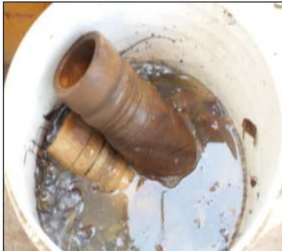
Figure 5: Bamboo Culms Soaked in Neem Leave Extract
