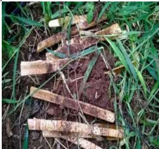
Figure 8: Termite test for split bamboo culms
